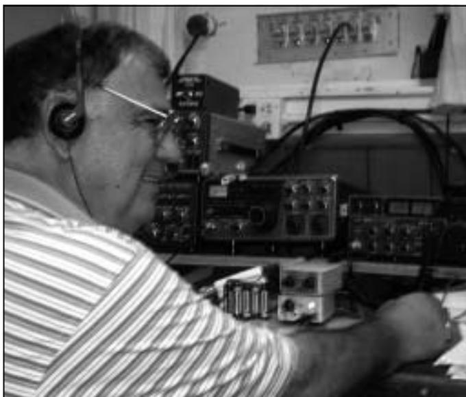
**ED, WA1ZCB AND HIS QRP SETUP: NOTE BATTERY PACK AND TUNER**
