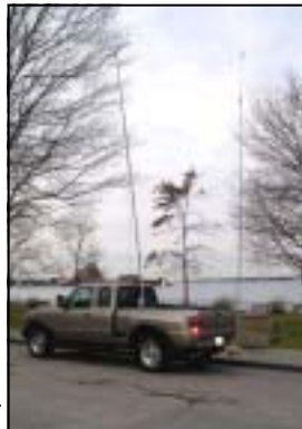
N1DT's F-150 REAR MOUNTED HOMEBREW 40/20 VERTICAL ANTENNA AND 2-M 4-EL YAGI
