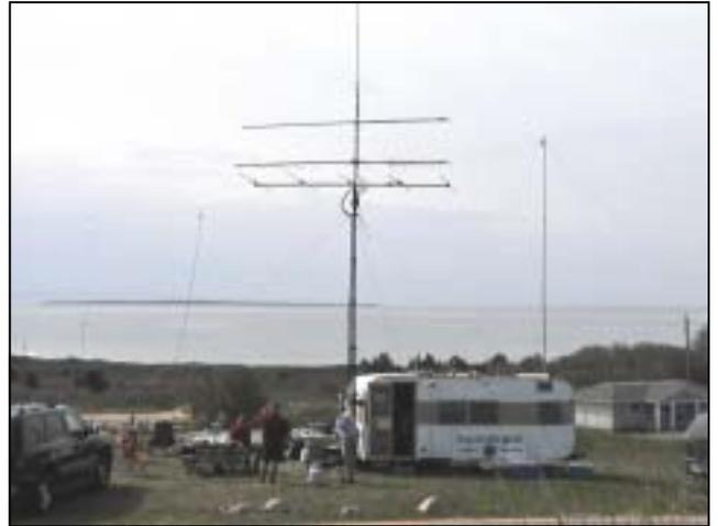
**N1JOY'S RADIO TRAILER WITH CRANK UP TOWER, YAGI'S FOR 6M, 2M, & 432 MHZ, AND A 500 FT. LONG WIRE. YOU CAN SEE NOMAN'S ISLAND OFF IN THE DISTANCE**
